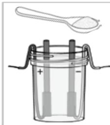
2. Dissolve 1 tsp soda in 100 ml water in the measuring beaker. Place the prepared graphite electrodes in the beaker. They must not touch each other.
