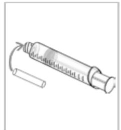
4. Cut off about 5 cm of the tube and put it over the tip of the third syringe.
