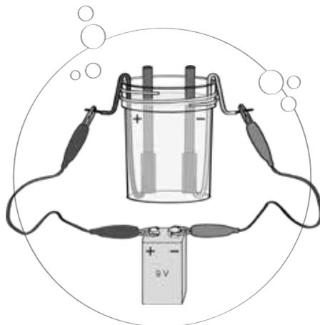
Electrolysis is a separation process of compounds. In the electrolysis of water, an electric current splits water into hydrogen and oxygen. Hydrogen rises at the negative pole (cathode). Oxygen rises at the positive pole (anode).
